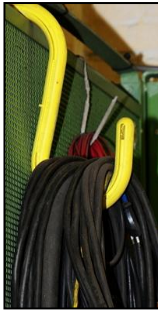
Place cords and cables into end of hook. Use hole in hook to secure with a zip tie, if needed.
