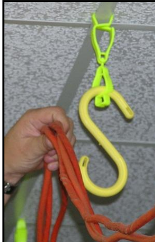
Place cords and cables into end of hook. Use hole in hook to secure with a zip tie, if needed.
