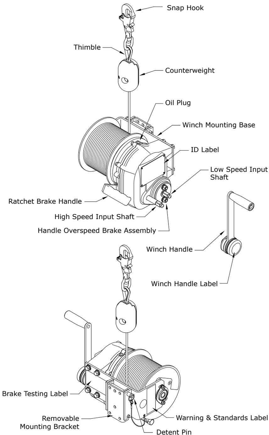
**Figure 2 - 8102001 Series Parts Identification**
